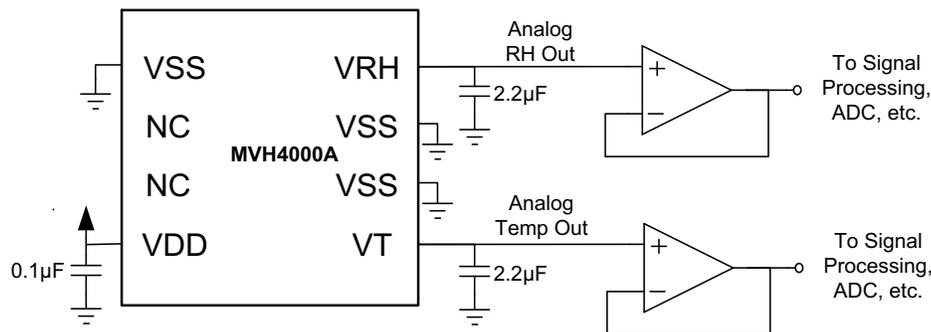
**Fig. 7: Application circuit to buffer relative humidity and temperature outputs.**
