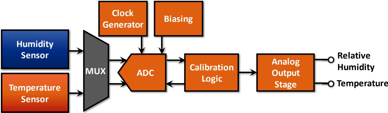
Fig. 4: MVH4000A series functional diagram.
