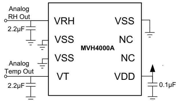
Fig. 3: Application Circuit.
