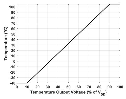
Fig. 9: Temperature vs. the VT output analog voltage.
