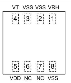
Fig. 1: Diagram of pin configuration (top view).
