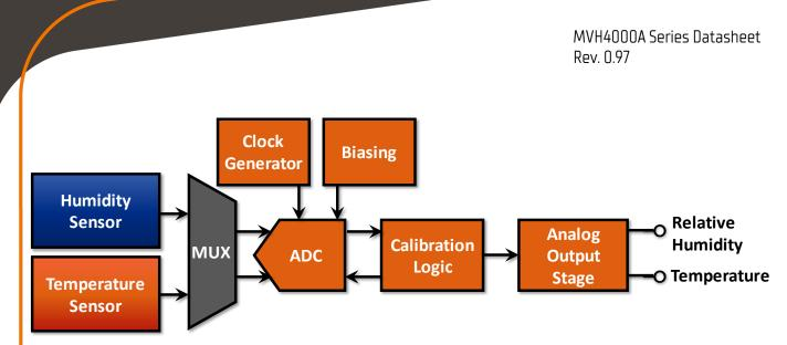
Fig. 4: MVH4000A series functional diagram.
