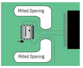
Fig. 14: Thermal isolation of sensor using milled PCB openings.
