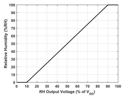
Fig. 8: Relative humidity vs. the VRH output analog voltage.
