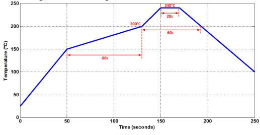
Fig. 13: Recommended lead-free soldering profile
