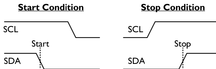
Fig. 8: I^2C bus start and stop conditions.
