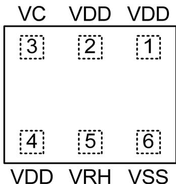
Fig. 1: Diagram of pin configuration (top view).
