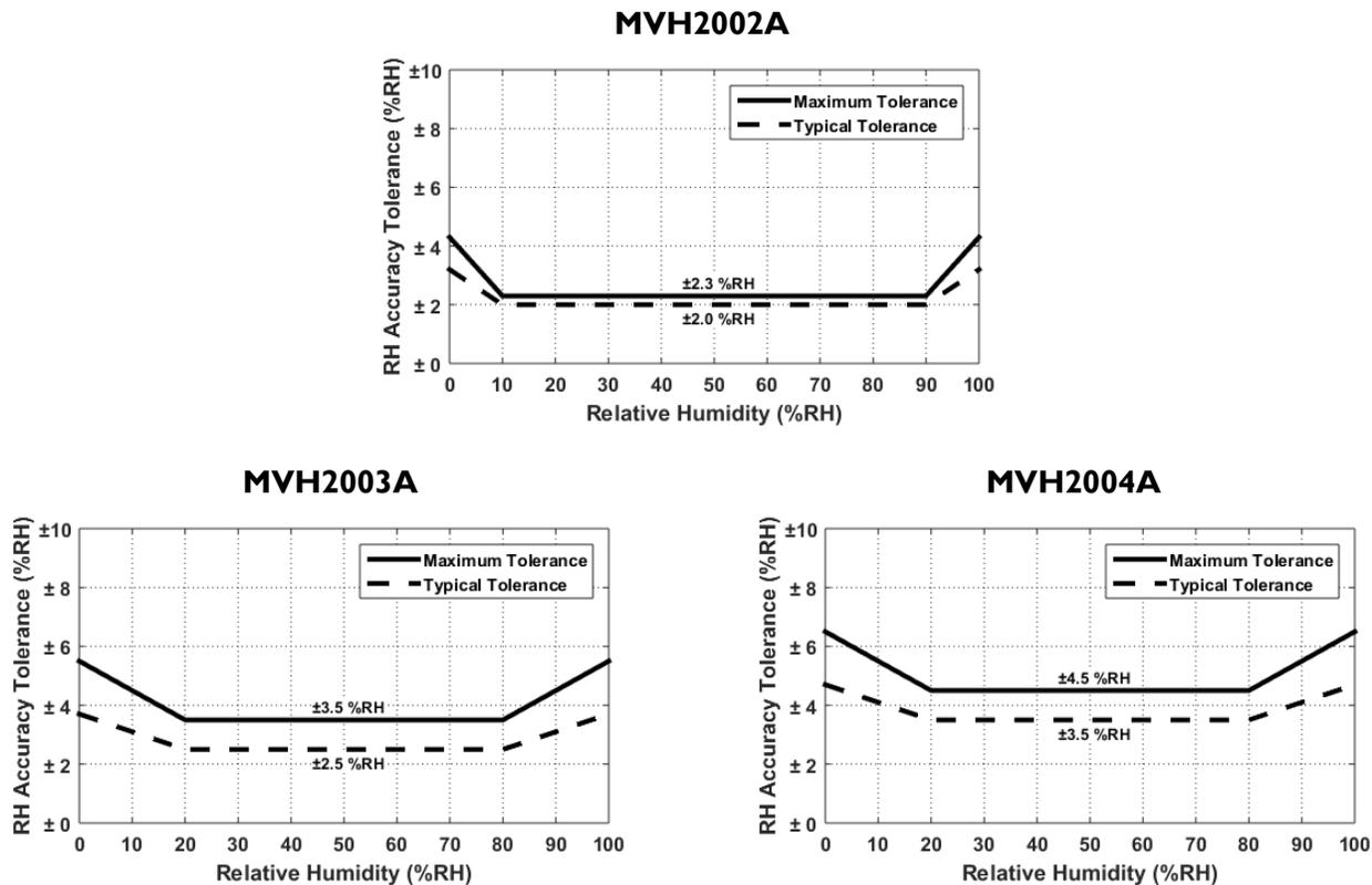
Fig. 5: Relative humidity tolerances at a temperature of +25°C.
